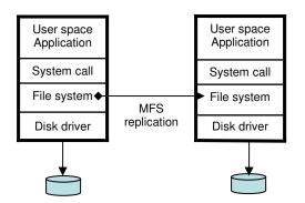
Figure 4: Mirror File System Replication
